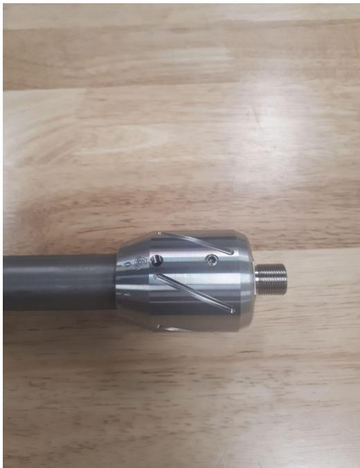
Screw tuner body onto tuner adaptor until the hex shoulder on the adaptor is slightly proud from the rim of the tuner body.
